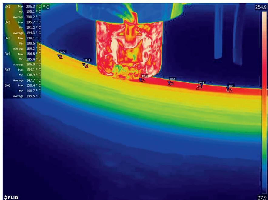
Thermal analysis of the deposited plastic strand in the large-format, extruder-based 3D printing process © Fraunhofer IWU
