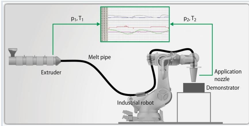
**Fig. 1.** The extruder is coupled to a flexible melt pipe with the print head fixed on the industrial robot © Fraunhofer IWU
