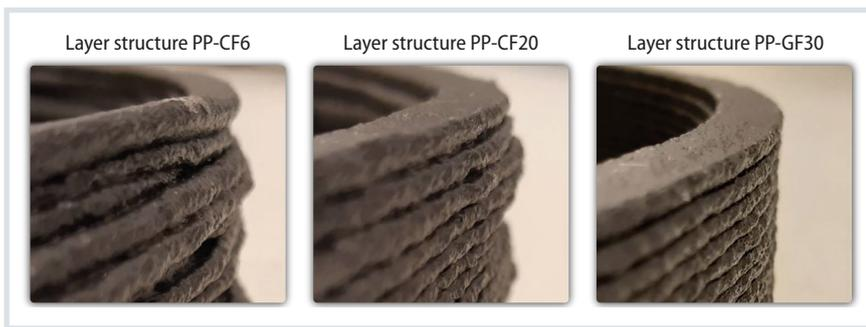
**Fig. 4.** The fiber length and the fiber content influence the layer stability and thus also the component quality © Fraunhofer IWU
