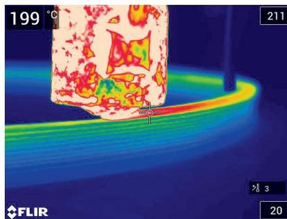
**Fig. 5.** The residual temperature of the deposited plastic strands fundamentally influences the component strength in the build direction (Z-direction) © Fraunhofer IWU
