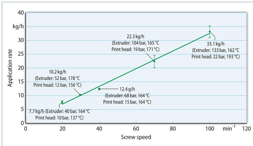
**Fig. 3.** The application performance of the Collin extruder (melt pipe DN16, printing nozzle 6 mm) has a linear deposition characteristic depending on the speed Source: Fraunhofer IWU; graphic: © Hanser
