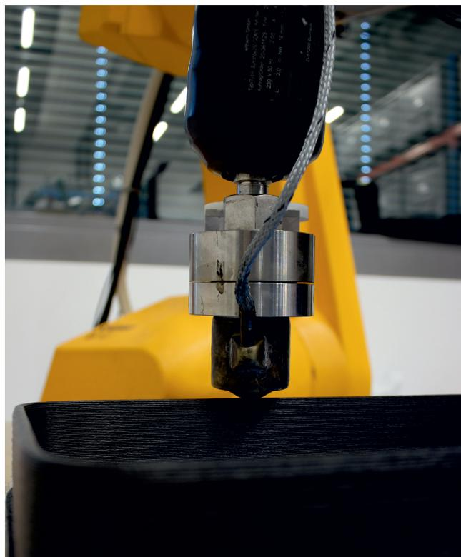
**Fig. 2.** The innovative print head permits pressure and temperature measurement of the plastic melt © Fraunhofer IWU
